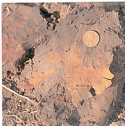
Figure 6. Examples of redox depletions. (A) A soil profile (Plinthaquic Paleudalf) showing well-developed redox depletions over 140 cm long in the B horizon. Iron depletions and clay depletions appear similar in photographs. In (B) gray Fe depletions (ID) occur primarily along ped surfaces as shown in this horizontal section at a depth of approximately 170 cm. Iron masses (IM) lie parallel to some depletions. In (C), clay depletions lie along ped surfaces (CD) and some root channels. The Fe masses (IM) occur in the matrix. Scale is in inches.
